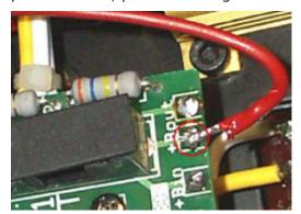
Next, solder the shorter red wire (as shown on the right) to the AutoBias board at the +B out as seen in the picture on the left. Run the longer red wire underneath the black Nichicon capacitor over to the area where the PhonoLogue card will be installed.
